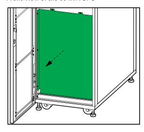
2. Install the batteries one string at a time and from the bottom and up.
