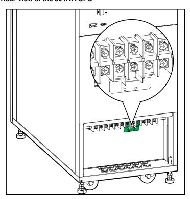
4. Route the power cables through the bottom of the UPS.
