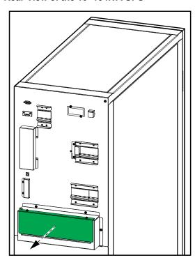
3. In dual mains systems, remove the single mains cable.
