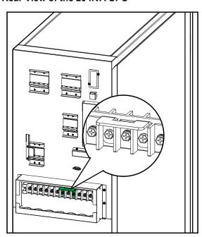
4. Route the power cables through the bottom of the conduit box.
