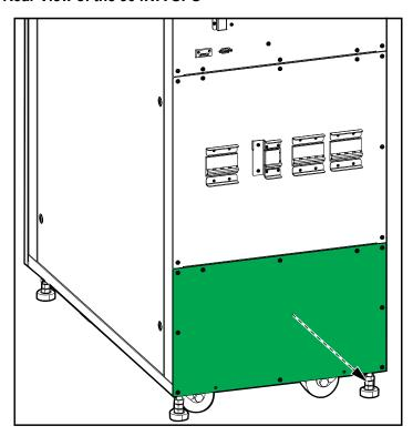
3. In dual mains systems, remove the single mains bracket.
