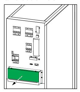
3. In dual mains systems, remove the single mains bracket.
