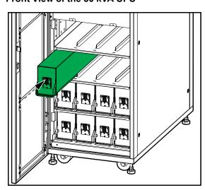
10–30 kVA 3:1 Install Batteries in the UPS
