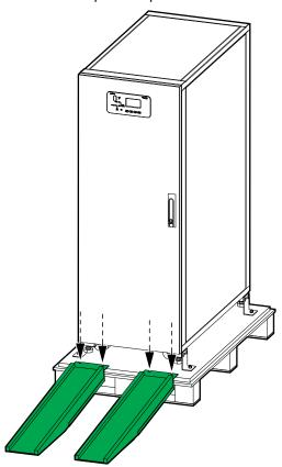
4. Loosen the bolts and remove the shipping brackets. Dispose of the shipping brackets.
